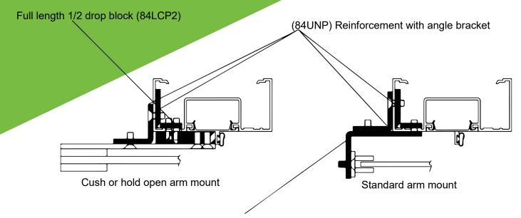
Alternate 1/2 drop angle bracket (84LCBR)
